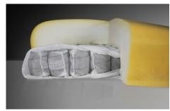
The PrimoComfort seat is designed with internal pocket coils with a cold-cure flexible polyurethane foam that shelters the springs and provides next-level relief and luxury. The molding process is fully water blown based and does not employ expanding agents (no CFC's).
